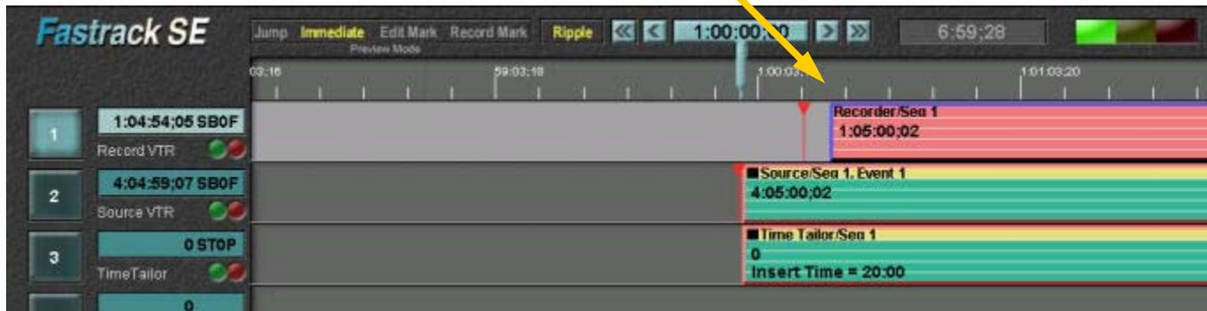
Press **[F3]** to start the Time Tailor process. You will see the Record and Source VTRs cue to their preroll positions, and the Current Position Indicator, “CPI”, (a red triangle on each track) move to the graphic representation of those positions. The machines roll (and the CPIs travel on the Timeline) toward the start of the Events on the Timeline.
