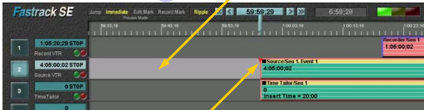
Press [N] to view the first frame of the Source Event. The CPI moves to the beginning of the Event on Track 2, and the monitor shows the first frame of the Source.
