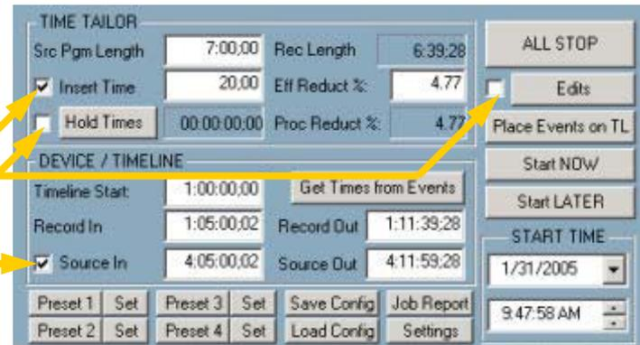
The "Src Pgm Length" field will be highlighted, with the contents ready to be replaced by whatever you type in. Type the length of the source material that is to be processed through the TimeTailor. Note that the ":" are entered automatically. Then press [Enter] (or enter a Source Out time after the Source In.)
