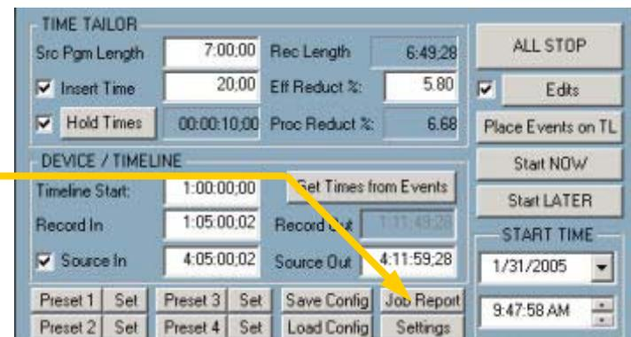
*A report can be generated for each set of data. It can be produced either before or after the Time Tailor process has been performed. Viewing the summarized report in the dialog window provides some key information that can be helpful in verifying the accuracy of the job parameters. To generate the report, [Click] on the “Generate” button.*
