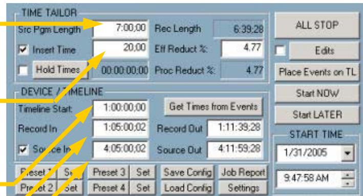
Running the Time Tailor process. This section will complete the basic “F1, F2, F3” Time Tailor task. We have completed the [F1] step, now for [F2] and [F3].
