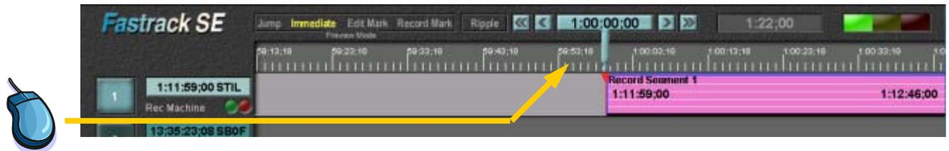
Note that when you [Click] on the Timeline scale, the Timeline mode is turned On. Remember to press [A] or All Stop to turn Timeline mode Off before continuing.
