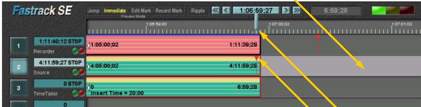
Press [Shift][N] (Search to Out Point). Notice the CPI on that Track moves to the end of the Event. And you see that frame on the monitor.
