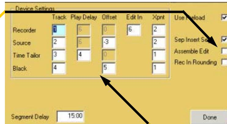
If there is additional delay in the path from the source VTR to the Record VTR, the settings need to be adjusted to compensate.
